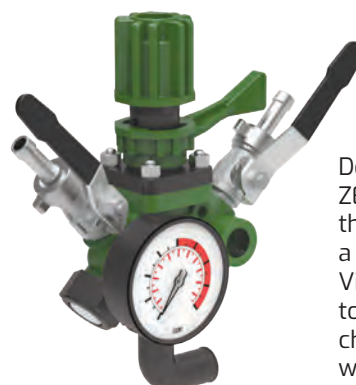
4900.14 27.0 GPM @ 350 PSI (2) 1/2" Hose Barb Outlets 3/4" Hose Barb Bypass Includes Pressure Gauge
