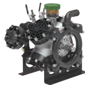
OMEGA 170 TS2C 46.0 GPM @ 725 PSI Shown with 1-3/8" 6-Spline Male PTO Thru Shaft Regulator / Control Unit is Included
