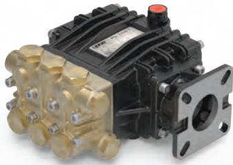
PN SERIES 0.5-4.0 GPM UP TO 2465 PSI Shown with SAE J609-A Flange for 3/4" Shaft Gas Engines Other drive options available
