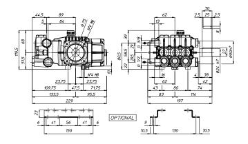
**Dimensional Drawings are** Shown in Millimeters. To Convert to Inches, Multiply Dimension x 0.03937
