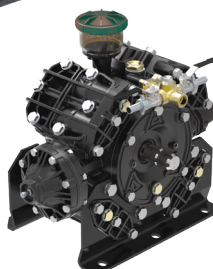
DELTA 170 TS2C 47.3 GPM @ 725 PSI Shown with 1-3/8" 6-Spline Male PTO Thru Shaft Other drive options available Regulator / Control Unit is Included
