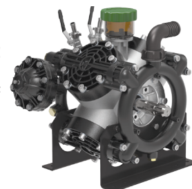
DELTA 170 TS2C 47.3 GPM @ 725 PSI Shown with 1-3/8" 6-Spline Male PTO Thru Shaft Other drive options available Regulator / Control Unit is Included
