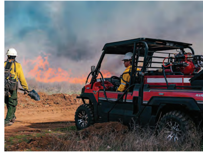
IOTA 25 GR3/4 7.0 GPM @ 300 PSI Shown with Gear Reduction for 3/4" Shaft Gas Engines Other drive options available Regulator / Control Unit is Included
