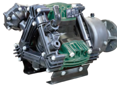
IOTA 25 GR3/4 7.0 GPM @ 300 PSI Shown with Gear Reduction for 3/4" Shaft Gas Engines Other drive options available Regulator / Control Unit is Included
