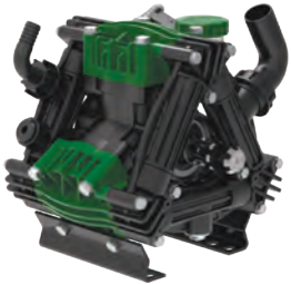
ZETA 120 1C 31.0 GPM @ 300 PSI Shown with 1-3/8" 6-Spline Male PTO Shaft Other drive options available
