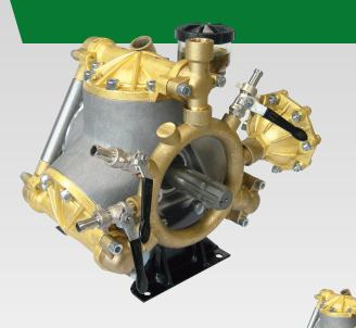
**BETA 110** 3-cylinder, high pressure, high volume diaphragm pumps are constructed of anodized aluminum, brass and stainless steel and have anodized aluminum, brass and stainless steel liquid handling parts. Includes mounting rails and control unit with pressure gauge. Simplicity of design and common parts allow for easy and economical maintenance.
