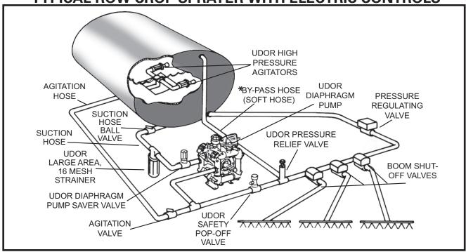
By-pass hoses must be open and unrestricted at all times. Never install an agitator on the by-pass line.
