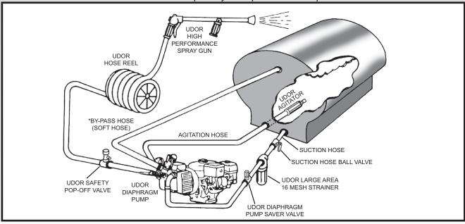
NOTE: All plumbing accessories should be the same or greater diameter as the feed line. All ball valves should be full port valves only.
