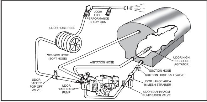
Bÿ-pass hoses must be open and unrestricted at all times. Never install an agitator on the by-pass line.
